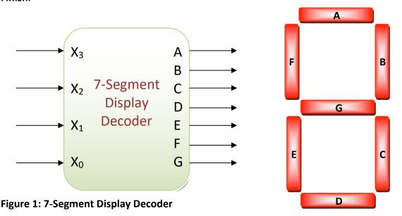
A 7-segment display is shown in **Figure 1**. The decoder provides the outputs A-G needed to light the proper segments of the 7-segment display based on a 4-bit input.
