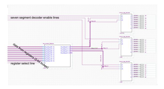
Part C is devoted exclusively to displaying the entered code to seven segment displays. The reg\_content\_Selector module takes the four two-bit buses from each of the registers (eight buses total) and uses a select line to choose which register's data is passed through. The Entry
