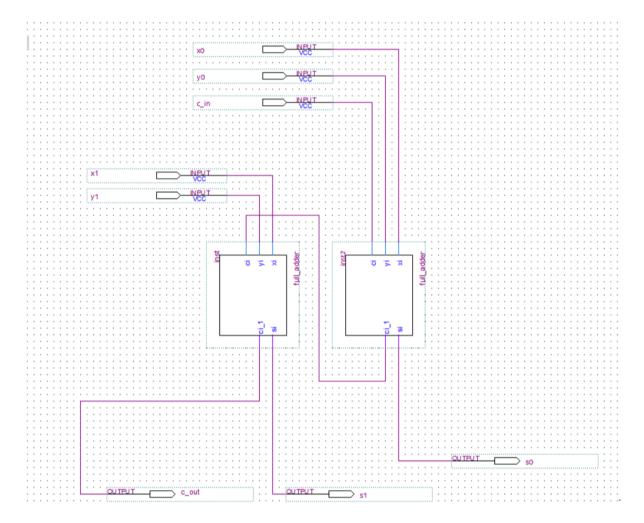
This module uses two full adders to create a ripple carry two-bit adder as seen in the textbook/lecture. First, x0 and y0 are added (along with the carry in), s0 is output, and the carry out is carried in to the next adder, which adds x1 and y1. This outputs s1 and the carry out signal.
