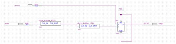
The effect of this circuit is to divide the clock frequency by 1024 two times (in this case, a 50 MHz clock) and synchronize the switch input with this. This fixes the signal for extended periods to prevent the anomalies that bouncing issues typically cause.
