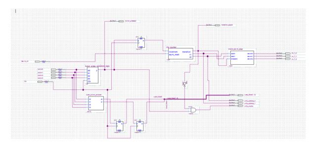
This is the module that reads and synchronizes all button inputs with the rest of the project.
