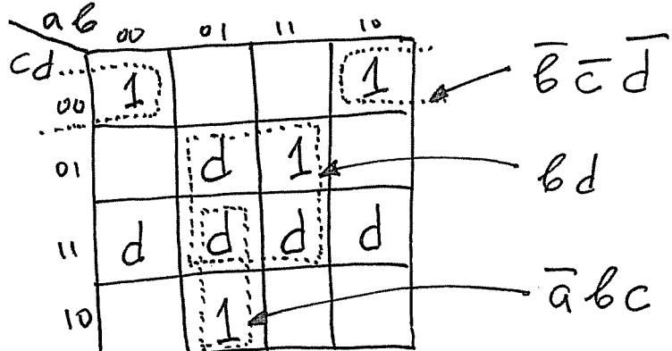
(b) Use the K-map to derive the minimum-cost SOP expression for the function F.
