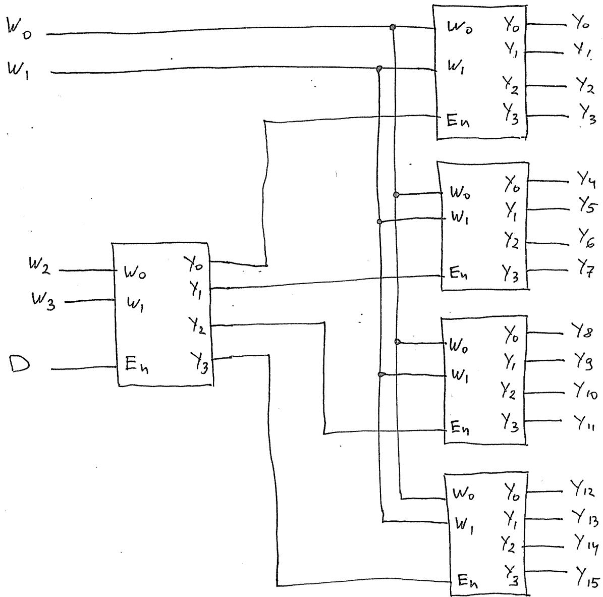
The enable input of the top-level decoder is used as the input data line.
