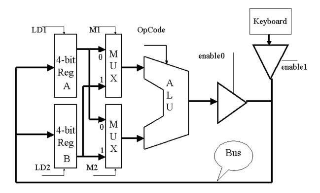
Describe what will happen when the clock arrives if the control signals are as follows for each case. Assume that the ALU block performs the following operations based on the OpCode input: 00 (ADD); 01 (SUB); 10 (AND) and 11 (OR)
