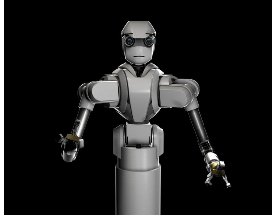
The upper torso humanoid robot is quipped with two arms and two webcams but only one of each will be used in this study.
