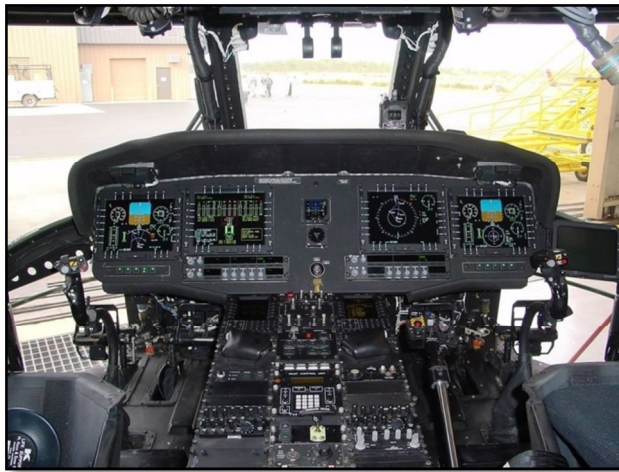
Figure 1. The many visual cues required to fly a UH-60 Black Hawk helicopter. Source: defenseindustrydaily.com .
