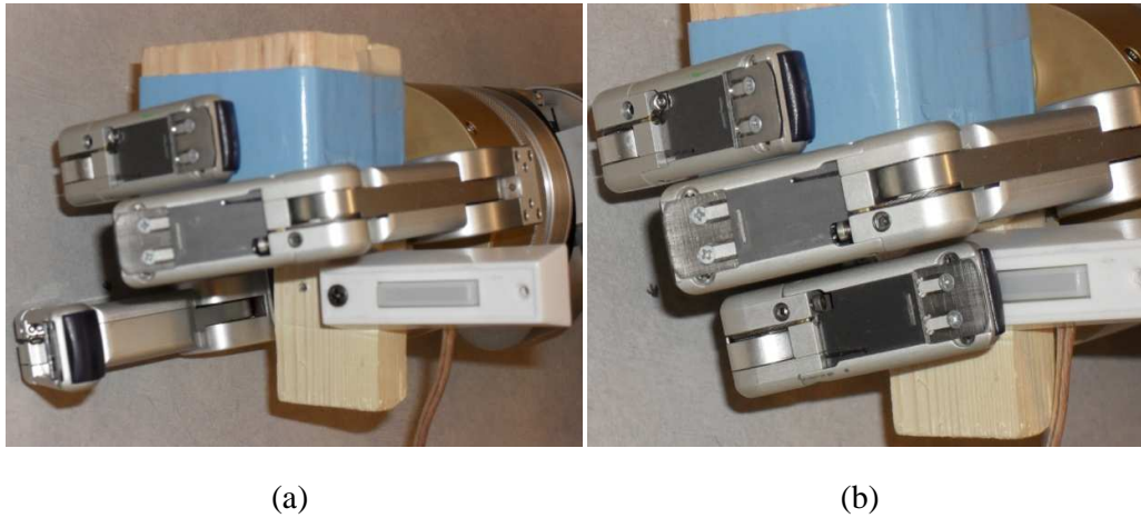
Figure 5. Portable device being grasped by the robot hand: (a) with finger 2 open; (b) with finger 2 closed.
