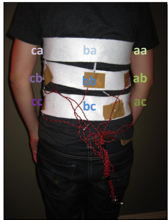
Figure 8. Final vibrotactile array configuration as worn by VFSS operator with location of array grids.
