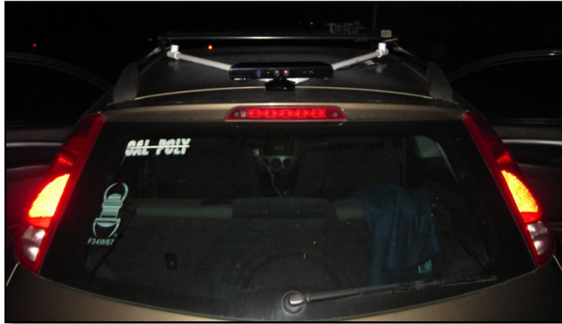
Figure 7. Microsoft Kinect as mounted on my 2000 Ford Focus for testing of the VFSS.
