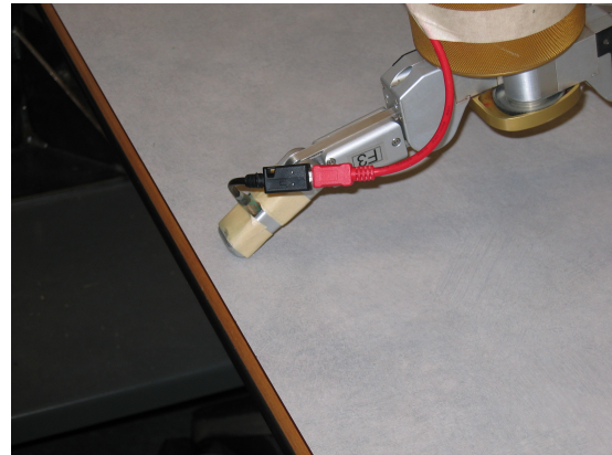
Figure 3: Robot finger with vibrotactile sensor exploring the table edge.
