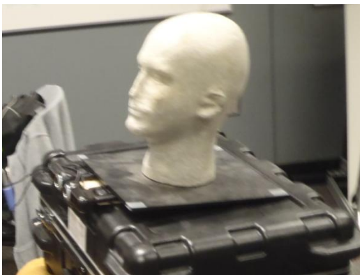
Figure 9 – Virtual head Manikin head sitting on top of dual Logitech Pro 9000 webcams is pictured. The webcams have built in speakers on either side which serve as the subjects' auditory modality.
