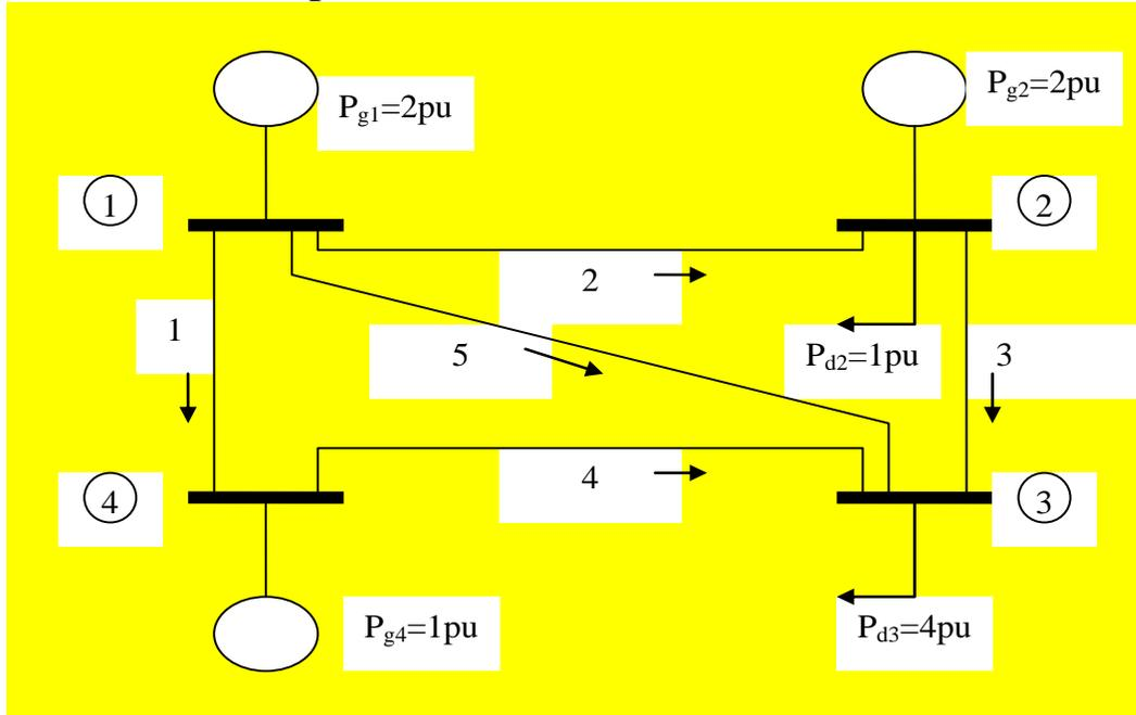
For example, the first column indicates that if we increase bus 1 injection by 1 pu, we get 0.3333 flowing over branches 1, 2, 5, with 0 pu on branches 3, 4<sup>1</sup>.
