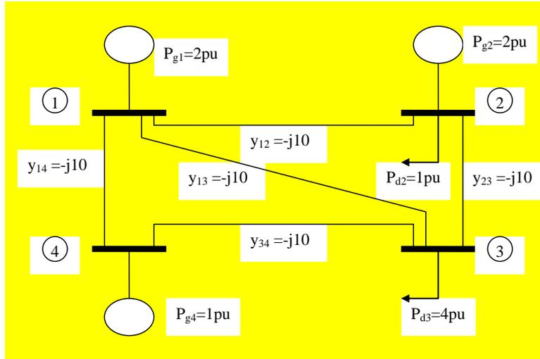
Fig. 2: Four-bus network used in example
