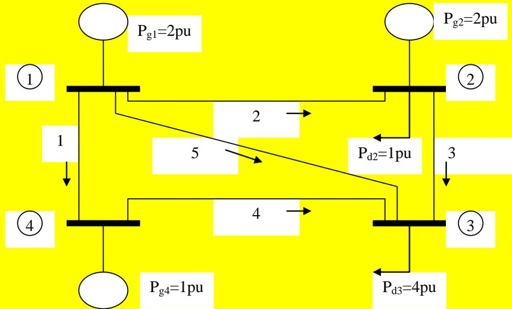
Fig. 6: Branches numbering for development of incidence matrix
