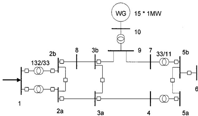
**Fig. 20.** Meshed system with wind farm.
