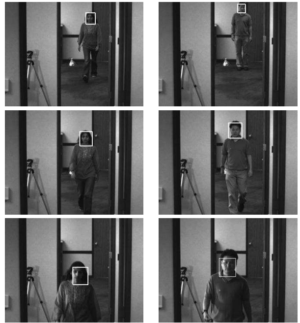
Fig. 2. Face tracking using PF-MT as the individuals walk through different lighting conditions. The white box shows the image region corresponding to MMSE estimate of the “shape vector”.
