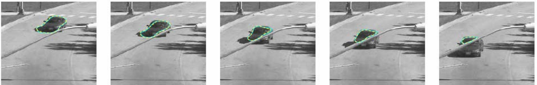
(a) Tracking the contour for the car to left of the pole using Algorithm 2
