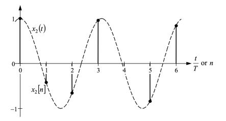
Figure 2:  $x_2(t)$  and  $x_2[n]$  in Example 2.
