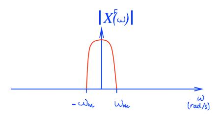
Figure 4: Spectrum of a lowpass CT signal x(t).
