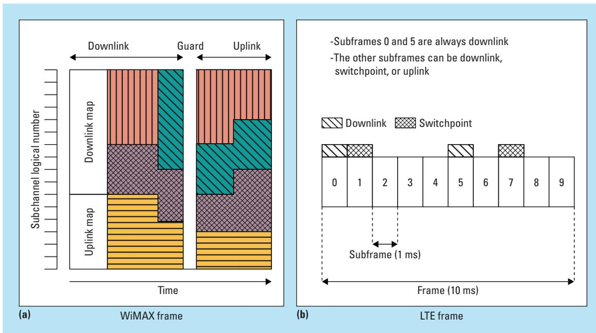
**Figure 2.** Both WiMAX and LTE employ reservation-based access using the concept of frames. Frames in (a) WiMAX (the different colors represent different users) and (b) LTE standards.
