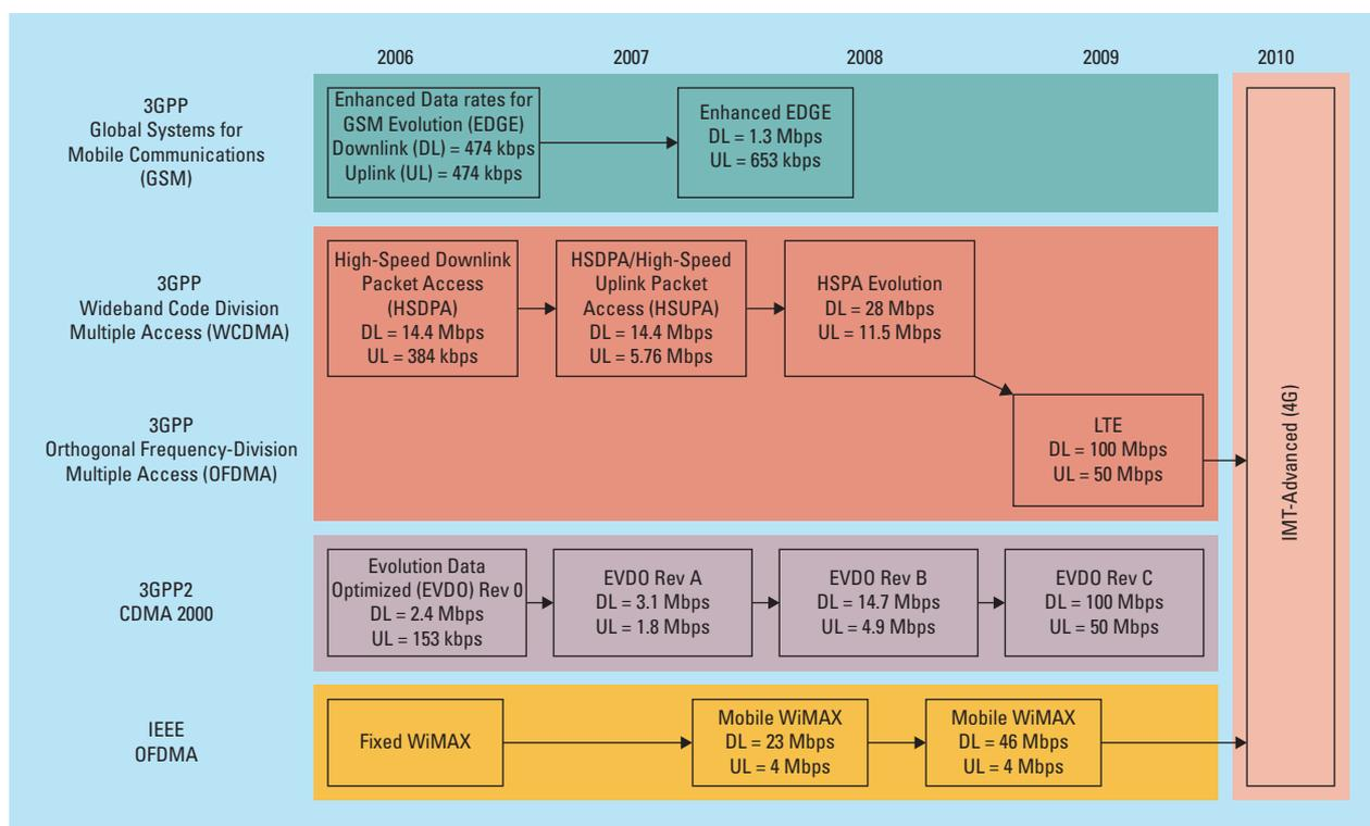
**Figure 1.** The Long-Term Evolution (LTE) and WiMAX standards' development. 3GPP2 is an organization structured similar to 3GPP. Evolution Data Optimized (EVDO) was developed to target IMT-2000 (3G) and is considered a predecessor of LTE.
