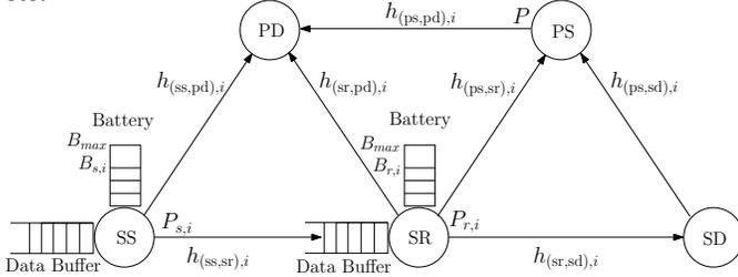
Fig. 1. Cooperative underlay cognitive radio system with energy harvesting.
