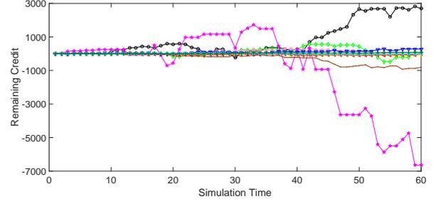
Fig. 3: Selected UEs' available credit vs simulation time with LCF user cooperation scheme.
