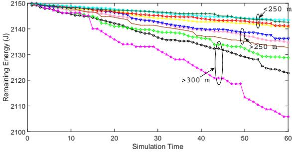
Fig. 2: Selected UEs' available energy vs simulation time with LCF user cooperation scheme.
