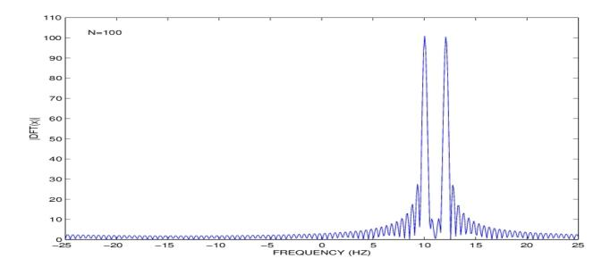
DFT with N = 100 and zero padding to 512 points. Resolved:  $F_2 - F_1 = 2 \text{ Hz} > 1/(NT) = 0.5 \text{ Hz}.$
