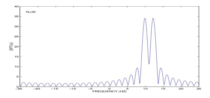
DFT with N = 30 and zero padding to 512 points. Resolved:  $F_2 - F_1 = 2 \text{ Hz} > 1/(NT) \approx 1.7 \text{ Hz}.$
