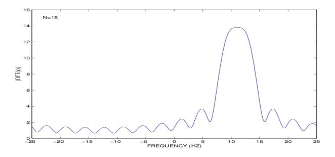
DFT with N = 15 and zero padding to 512 points. Not resolved:  $F_2 - F_1 = 2$  Hz  $< 1/(NT) \approx 3.3$  Hz.
