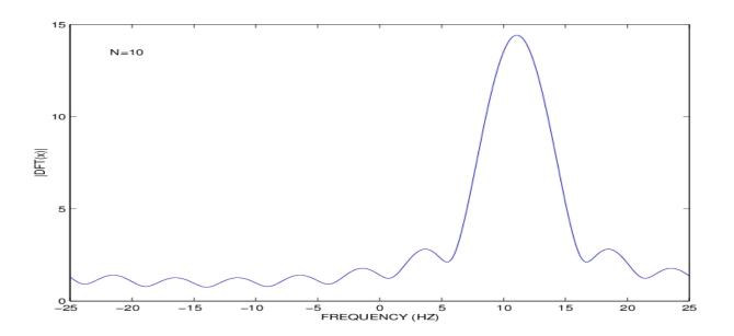
DFT with N = 10 and zero padding to 512 points. Not resolved:  $F_2 - F_1 = 2 \text{ Hz} < 1/(NT) = 5 \text{ Hz}.$
