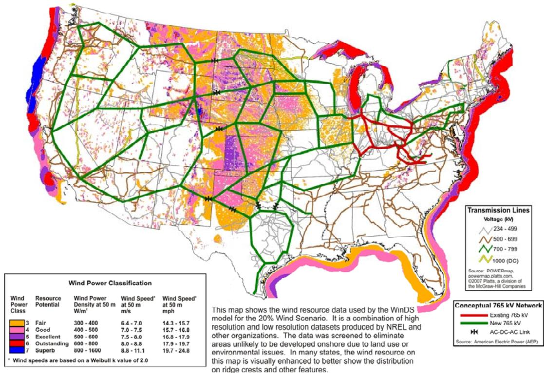
Fig. 15c: AEP's conceptual for moving wind energy
