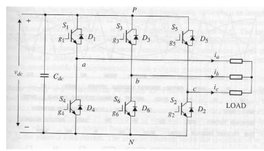
The inverter is connected to a three phase balanced RL load, and its DC voltage is 1220 volts. The inverter is modulated by space vector modulation and its simulation algorithm is given in the figure below ("Table 4-4" is the table to the right).
