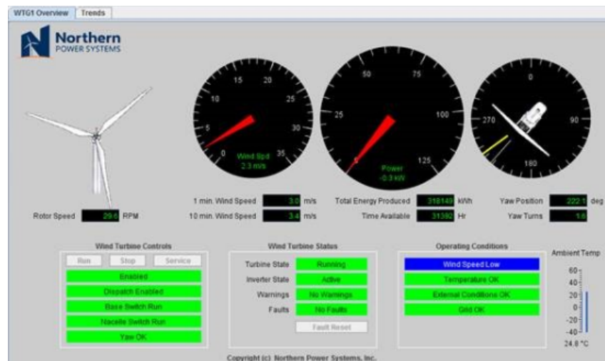
Figure 1.7: SCADA interface of the 100 kW wind turbine on the Iowa State University campus. Interact online at https://smartview.northernpower.com/fleet.php ; “studentview@iastate.edu, isuwind”.
