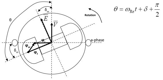
"At t=0 the phasor V is located at the axis of phase a, i.e., at the reference axis in Figure 4.1. The q axis is located at an angle  $\delta$ , and the d axis is located at  $\theta = \delta + \pi/2$ .
