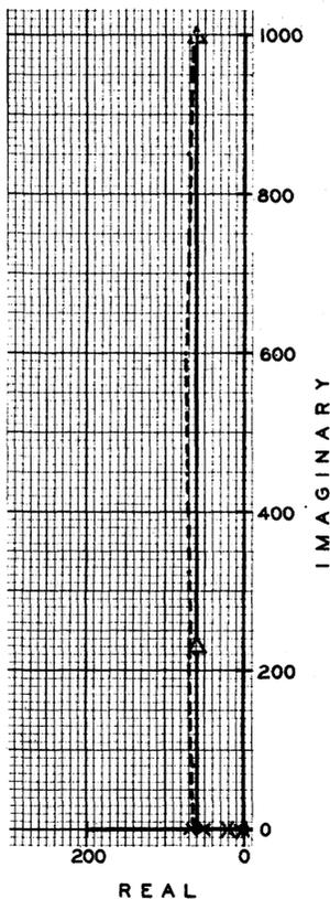
Fig. 7B. Root locus plot for excitation system with rate feedback.
