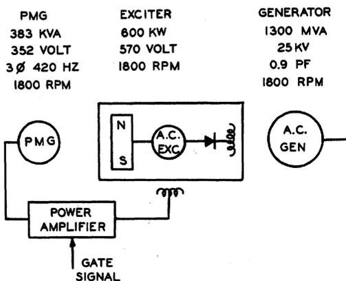
Fig. 2. Schematic of rotating exciter, PMG, generator, and regulator.
