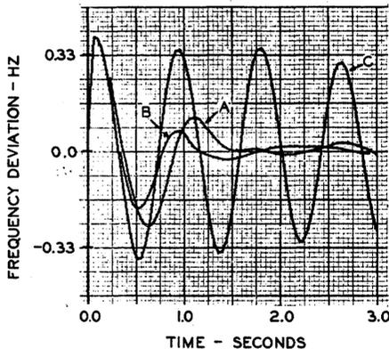
Fig. 9. Frequency deviation comparison for a 4-cycle fault on the Midway circuit adjacent to the 500 kV bus at the Diablo Canyon Site.
