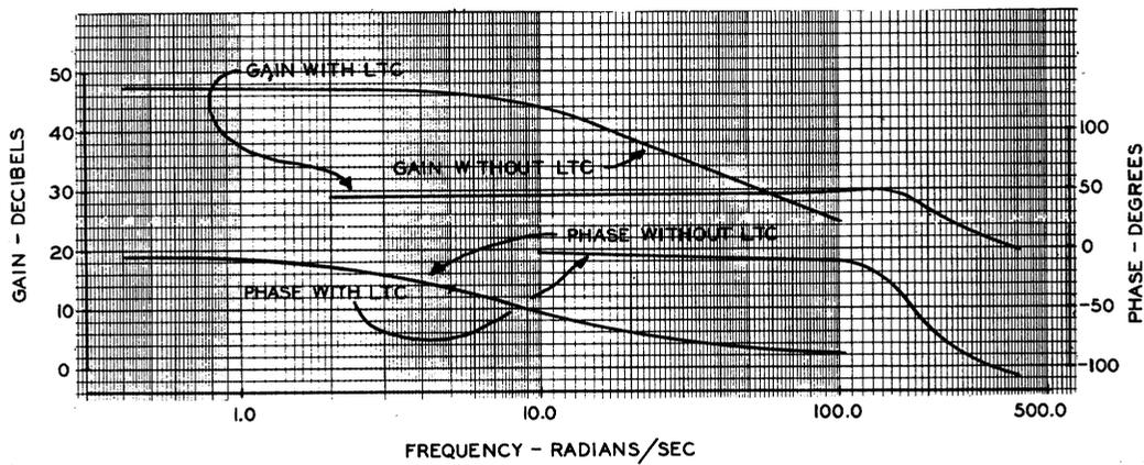
Fig. 4. Frequency response tests for exciter, with and without low time constant compensation.
