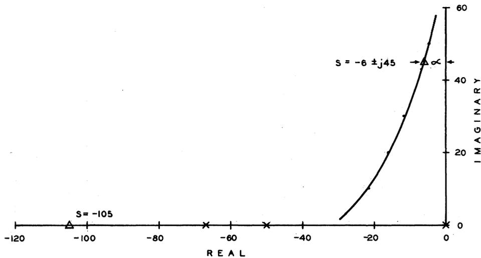
Fig. 7A. Root locus plot for excitation system and generator closed loop without rate feedback.
