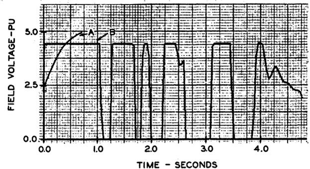
Fig. 11. Field voltage comparison for a 9.6-cycle fault on the Midway circuit adjacent to the 500 kV bus at the Diablo Canyon Site.
