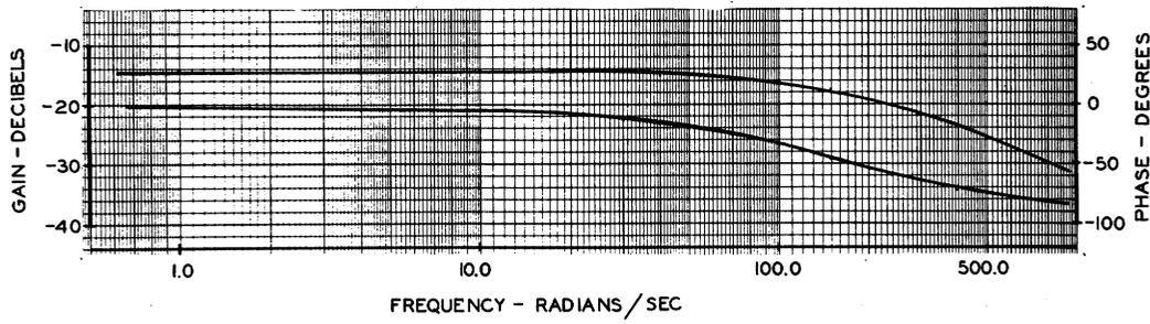
Fig. 3. Frequency response of the regulator error sensing filter.
