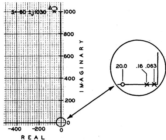
Fig. 7C. Root locus plot for excitation system and generator closed loop with rate feedback.
