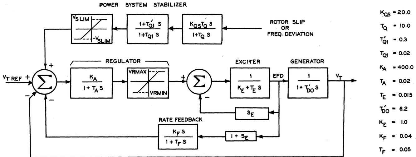
Fig. 1. Excitation and power system stabilizer block diagram with tabulation of design values.
