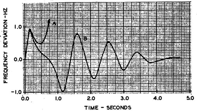
Fig. 10. Frequency deviation comparison for a 9.6-cycle fault on the Midway circuit adjacent to the 500 kV bus at the Diablo Canyon Site.
