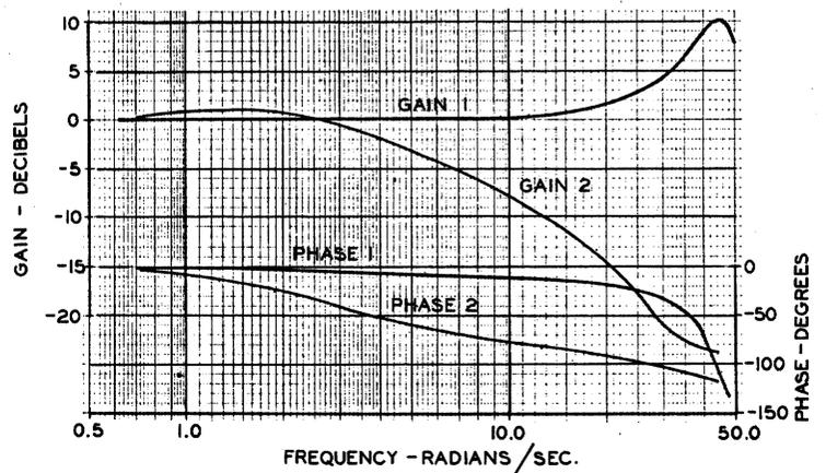
Fig. 6. Frequency response comparison of the excitation-generator closed loop with and without rate feedback.
