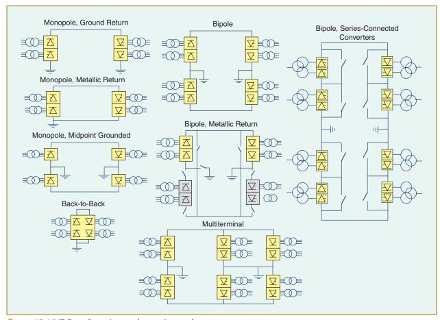
figure 13. HVDC configurations and operating modes.
