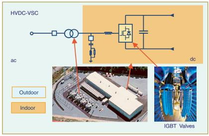
figure 4. HVDC with voltage source converters.
