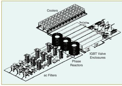
figure 15. VSC HVDC converter station.
