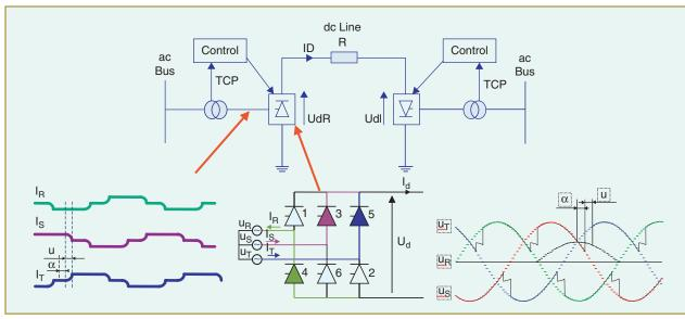
figure 16. Conventional HVDC control.
