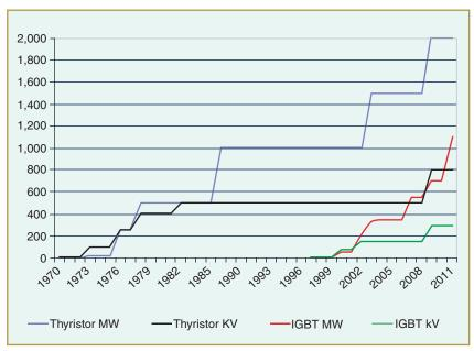
figure 8. Solid-state converter development.
