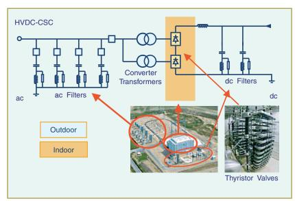
figure 3. Conventional HVDC with current source converters.
