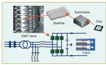
figure 9. HVDC IGBT valve converter arrangement.
