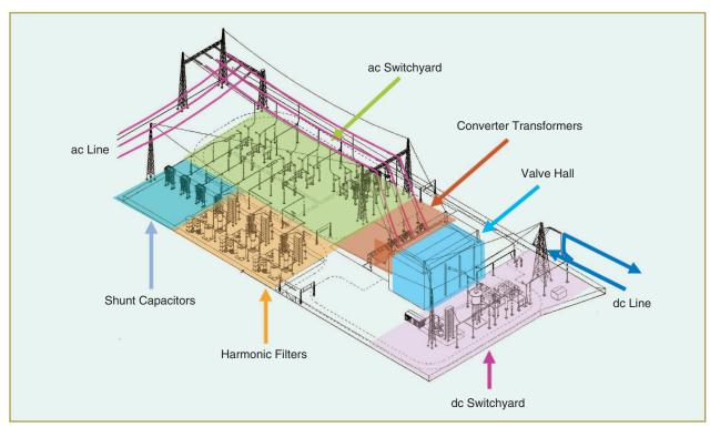
figure 14. Monopolar HVDC converter station.
