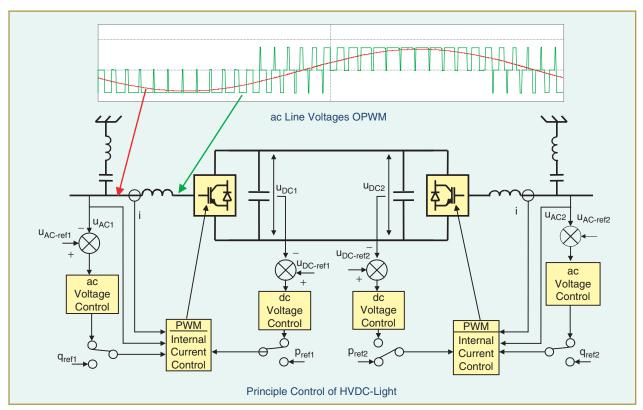
figure 17. Control of VSC HVDC transmission.
