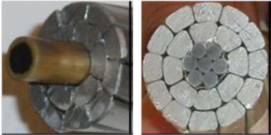
Figure B.13 Composite-core Cables. Left: ACCC. Right: ACCR [96]
