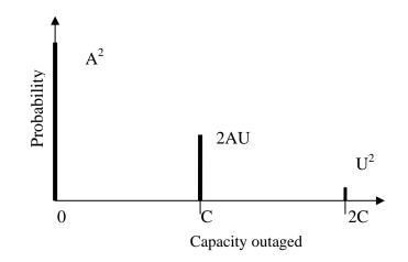
Fig. U19.5: pmf for Capacity Outage of 2 Unit Example
