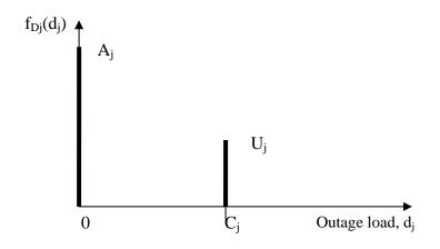
Fig. U19.20: Two state generator outage model
