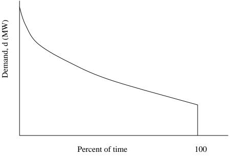
Fig. U19.12: Load duration curve
