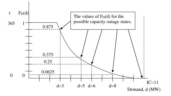
Fig. U19.14: Load shape curve for example
