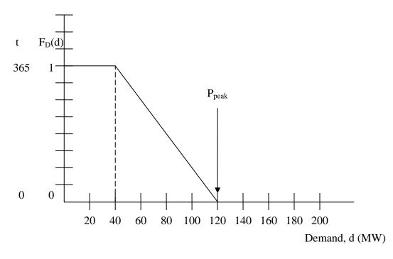
Fig U19.15a: Load shape curve for example [1] The procedure of the previous section was applied, i.e., the following expression was evaluated,
