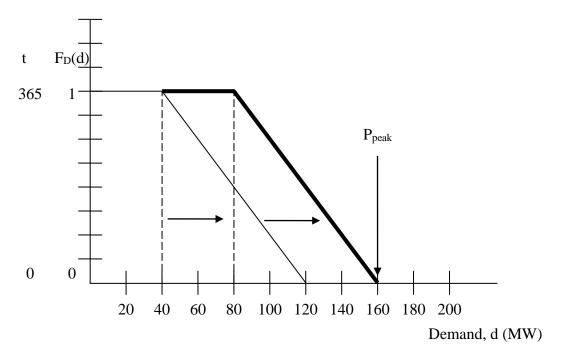
Fig U19.15b: Load shape curve for example [1]
