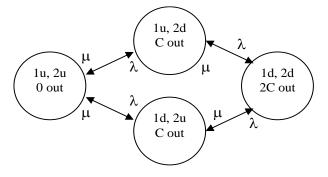
Fig. U19.6: State Space Model for 2-Unit System
