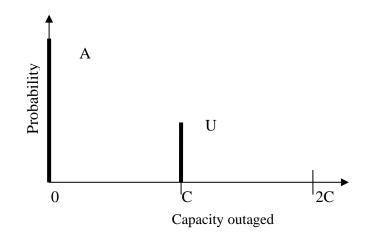
Fig. U19.3: pmf for Capacity Outage of One-Unit Example
