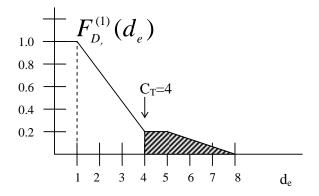
Fig. U19.23: Illustration of loss of load region
