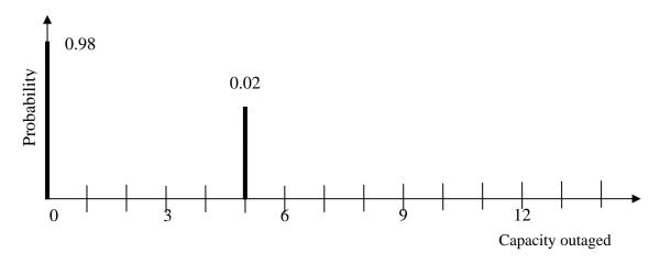
Fig. U19.9: pmf for 5 MW Capacity Outage
