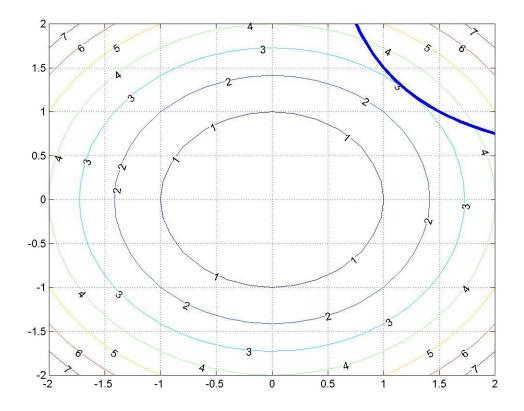
Fig. 3: Contour plots with equality constraint From the plot, we see that the solution is about  $(x_1, x_2)_0 \approx (1.25, 1.25)$ , as this point results in the smallest possible value of *f* that is still on the equality constraint. The value of *f* at this point is 3. We will check this analytically in the next section.
