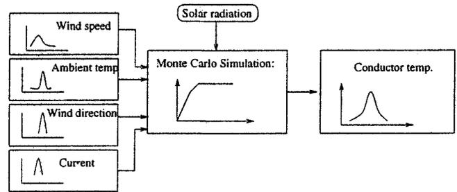
Fig. 6. MC simulation for conductor temperature.
