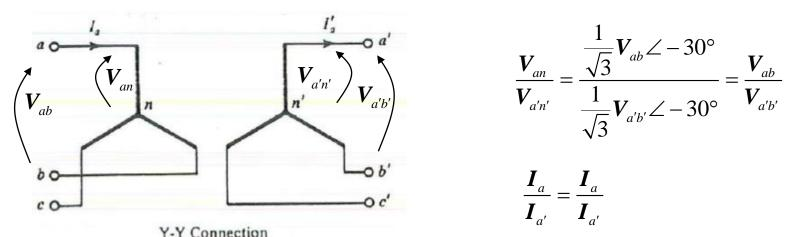
This means that the ratio of the line-to-line voltages on either side equals the ratio of the line-to-neutral voltages on either side if we can convert the transformer to an "equivalent Y-Y."
