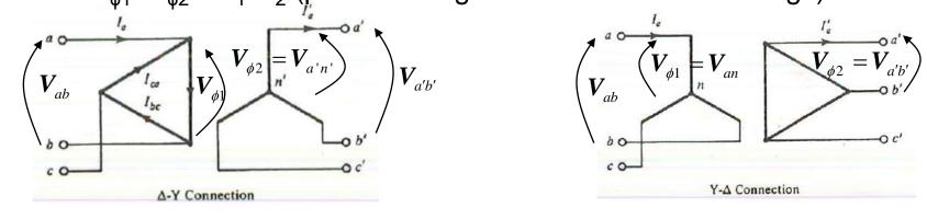
$$\frac{V_{ab}}{V_{a'b'}} = \frac{V_{\phi 1}}{\sqrt{3}V_{a'n'} \angle 30^{\circ}} = \frac{V_{\phi 1}}{\sqrt{3}V_{\phi 2} \angle 30^{\circ}} = \frac{N_{1}}{N_{2}} \frac{1}{\sqrt{3}} \angle -30^{\circ} \qquad \frac{V_{ab}}{V_{a'b'}} = \frac{\sqrt{3}V_{an} \angle 30^{\circ}}{V_{\phi 2}} = \frac{\sqrt{3}V_{\phi 1} \angle 30^{\circ}}{V_{\phi 2}} = \frac{V_{\phi 1}}{V_{\phi 2}} \sqrt{3} \angle 30^{\circ} = \frac{N_{1}}{N_{2}} \sqrt{3} \angle 30^{\circ}$$
