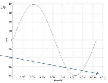
Since 1 cycle completes  $2\pi$  radians,  $\omega=(2\pi \text{ rad/cyc})*60\text{cyc/sec}=377\text{rad/sec}$ . We can therefore express this voltage
