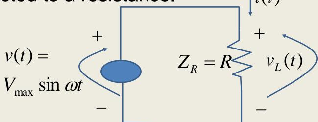
We apply Kirchoff's Voltage Law (KVL): the sum of voltages around the loop must be 0:  $v(t) - v_{I}(t) = 0$
