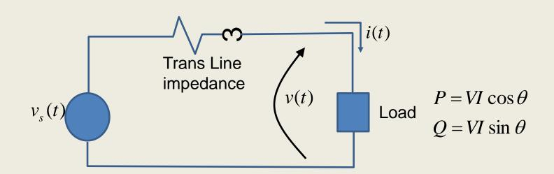
Assume V is constant, and we must supply P (this is the real power of the load). With V and P constant, from  $P=VIcos\theta$ ,  $Icos\theta=I\times pf$  must be constant. What do we want pf to be?
