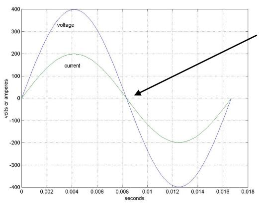
Current & voltage cross 0 simultaneously
