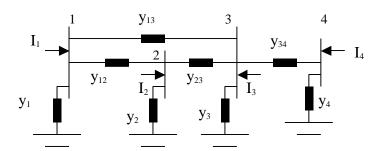
Fig. T7.4: Network for Motivating Admittance Matrix
