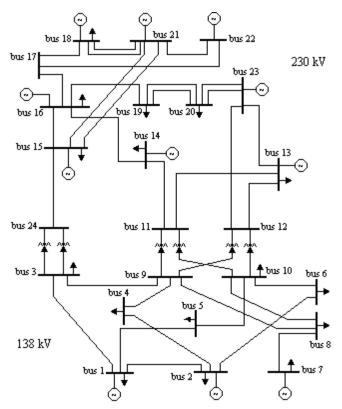
Figure T7.9 – The IEEE Reliability Test System [12]
