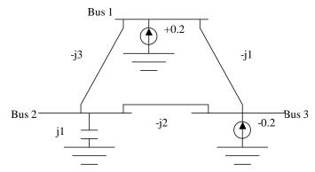
2. Form the Y-bus for the following two-bus power system, in both rectangular and polar notation. The reactance  $X_{12}$  is given in per unit.
