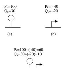
Fig T7.3: Illustration of (a) positive injection, (b) negative injection, and (c) net injection
