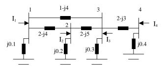
Fig. T7.5: Circuit for Example T7.1
