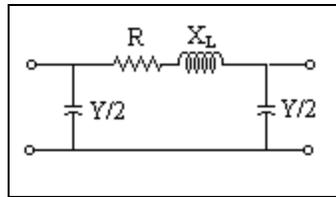
Figure T1.1 Pi-Equivalent Model of a Transmission Line
