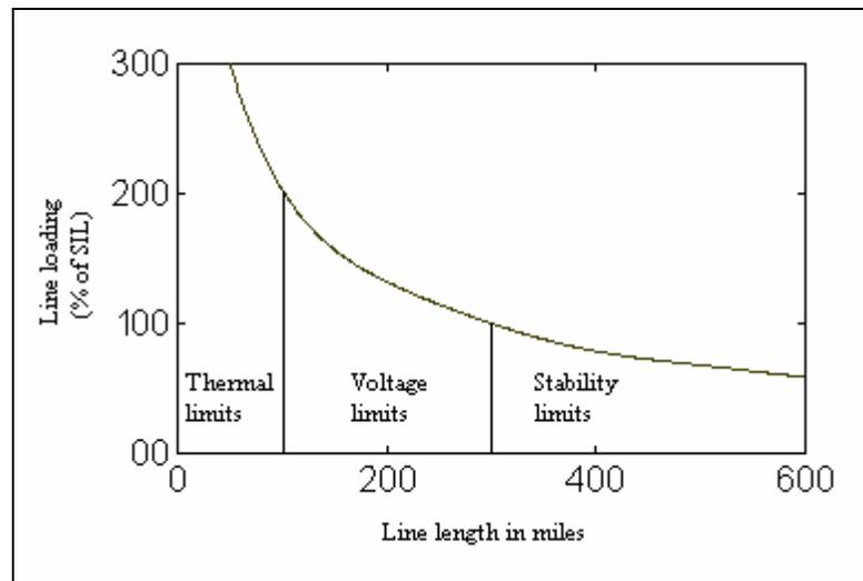
Figure T1.4 Line Loadability in Per-Unit SIL as a Function of Line Length
