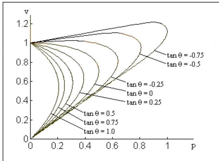
Figure T1.3 Plot of  $v$  vs.  $p$  for Various Values of Power Factor
