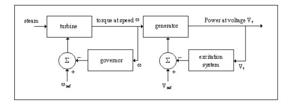
Figure G1.1 Block Diagram for Turbine-Generator System
