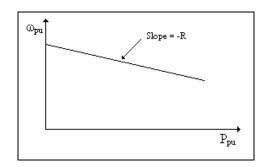
Figure G1.15 Steady-State Droop Characteristic
