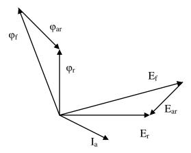
Figure G1.4 Phasor Diagram for Synchronous Machine
