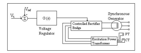
Figure G1.12 Static Type Excitation System
