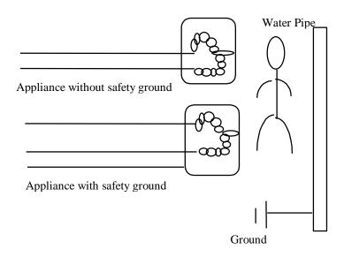
Figure D1.10 Safety Ground Principles
