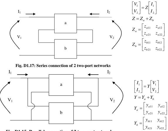
Fig. D1.15: Parallel connection of 2 two-port networks
