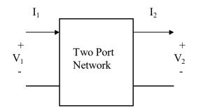
Fig D1.13: Generalized two port network with I<sub>2</sub> direction reversed
