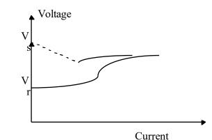
Figure D1.2 Voltage Current Characteristics of SiC Gapped Arrestor
