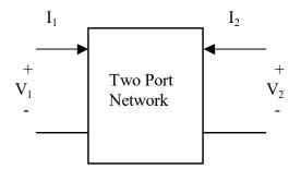
Fig. D1.12: Generalized Two-Port Network
