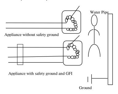
Figure D1.11 Application of Ground Fault Interrupter
