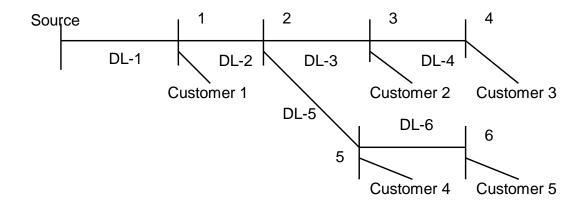
Figure D1.6 Multiple Branch Distribution System
