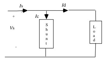
Figure D1.7 Shunt Compensation
