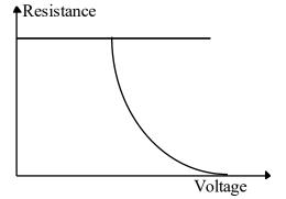
Figure D1.1 Lightning Arrestor Impedance Model
