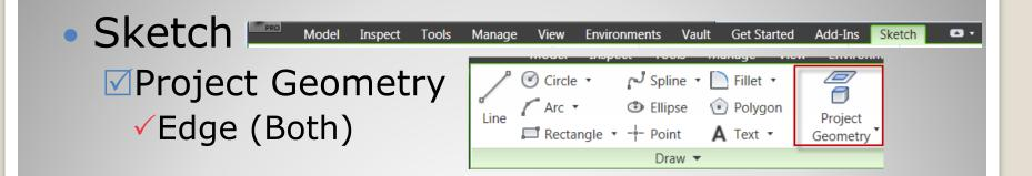
Important: Project Geometry allows the edges to be used in the sketch. This will be used to make new features concentric to the edges.
