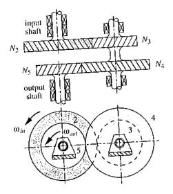
**Input and output shafts are coincident—lined up on the same axis.** This is a two stage reverted train—note that the center distance of stage 1 must be equal to the center distance of stage 2
