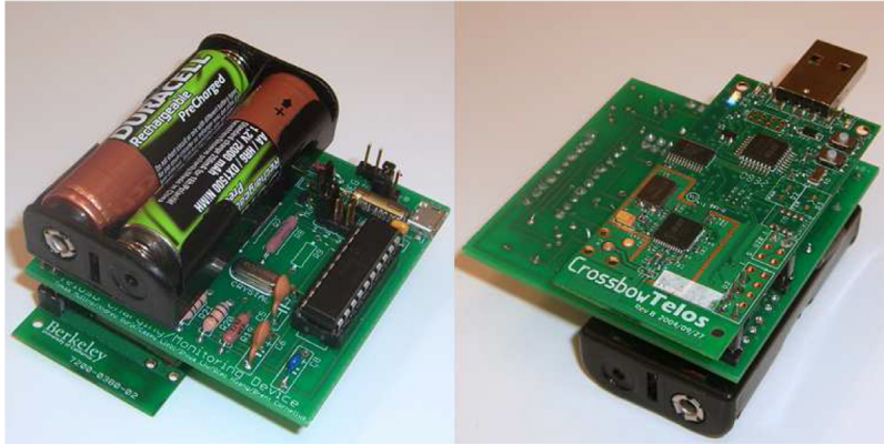
Fig. 8. TelosB power meter kit used in LBA. The operation power consumption of the kit is 2.4 \mu W which is small compared to regular TelosB power consumption.
