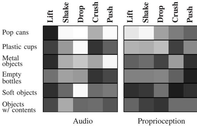
Fig. 6. Success rates for the odd one out task, shown for each category, and for each behavior-modality context. Light color indicates high success rates, while dark color indicates low success rates.
