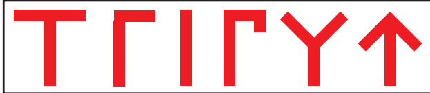
Fig. 2. The six different tools used by the robot. From left to right: T-Stick, L-Stick, Stick, L-Hook, Y-Stick, Arrow.
