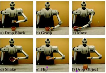
Figure 1: The six exploratory behaviors performed by the robot. Before each trial the block and one of the twenty objects were placed at marked locations on the table. The robot performed each behavior in the order shown after it grasped the block and positioned its arm in the area above the object.
