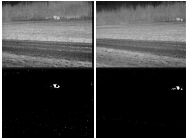
Fig. 5.2. Frame 160 and 250 of a moving vehicle IR sequence along with detected objects (sensor recovering after panning motion)
