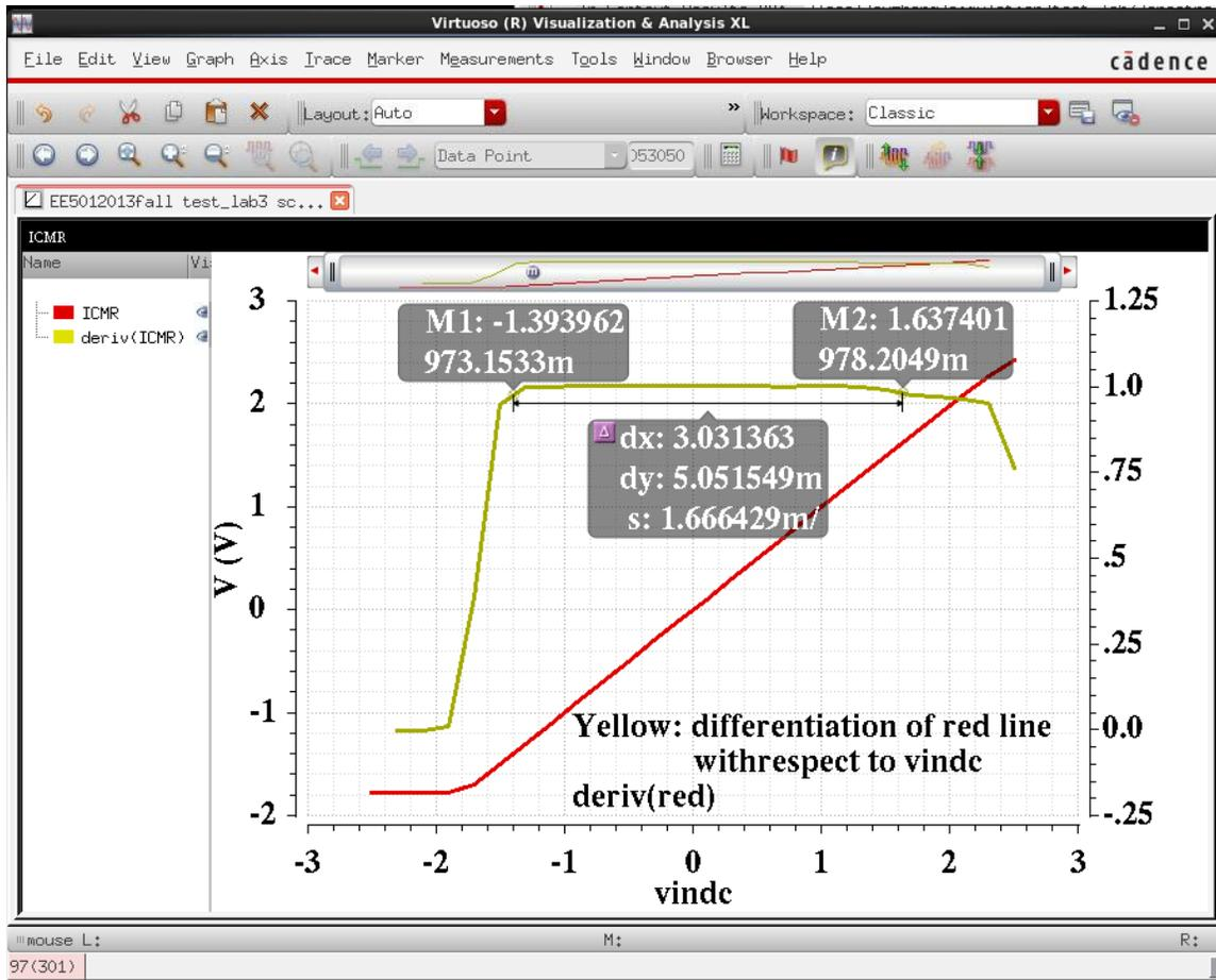
Fig. 7 ICMR of the designed amplifier
