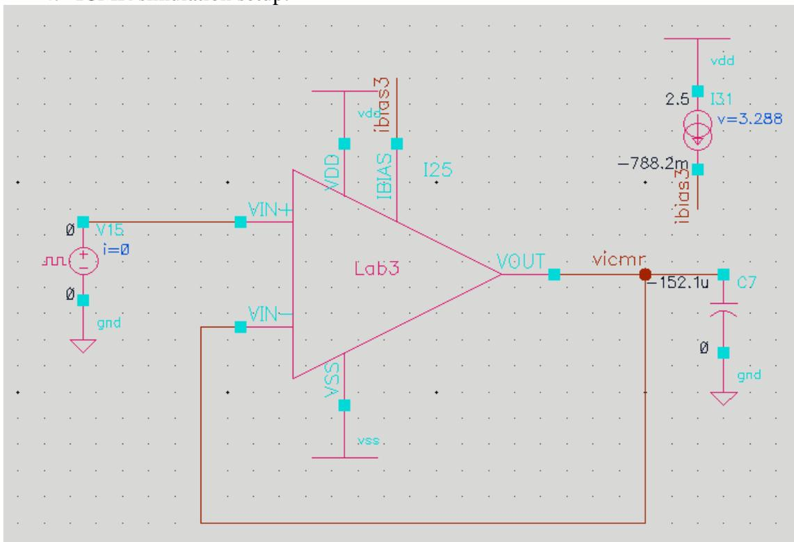
Fig. 6 ICMR simulation setup
