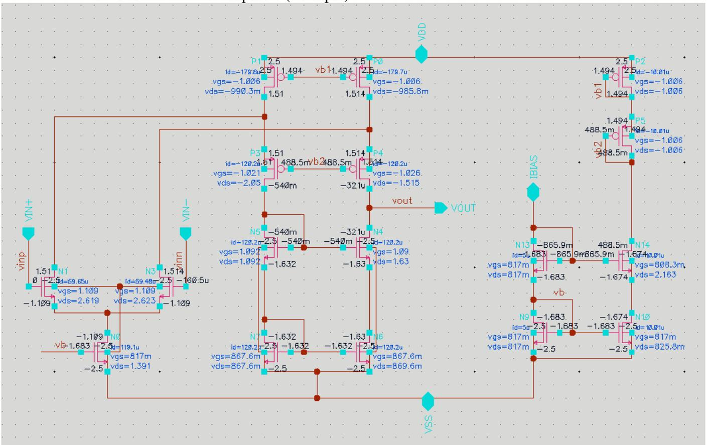
Fig. 1 Folded-cascode amplifier example
