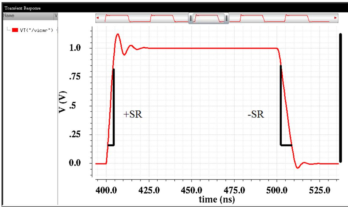
Fig. 9 Slew Rate simulation results
