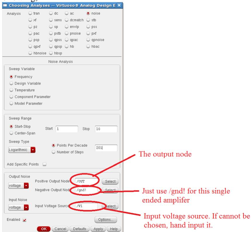
Fig. 11 "noise" simulation setup
