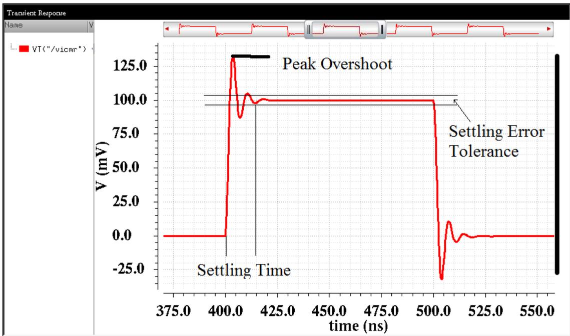
Fig. 10 Overshoot and settling time simulation results
