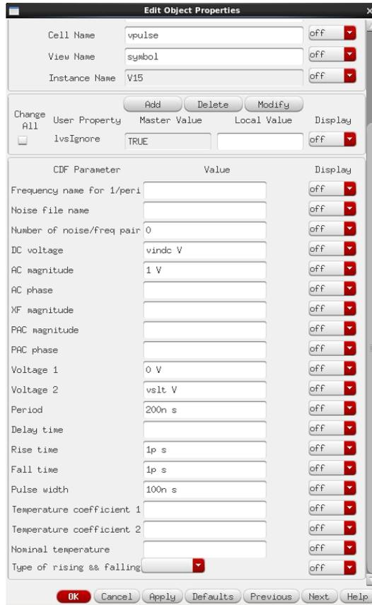
Fig. 8 “vpulse” setup for slew rate and overshoot simulations
